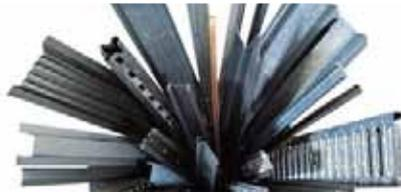
Metal is usually separated into two groups: aluminum and steel. You can test which metal your waste is by using a magnet. Aluminum metal is non-magnetic whereas steel is magnetic.
